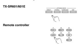
**DIRECT:** Changes the listening mode for the signal type that is currently being input from the selected input source to the Direct listening mode. If pressed, the corresponding settings in the "Input Setup" menu for the selected input source is also changed (see page 54).
